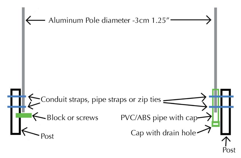
Setting the pole on a slight angle (10-20 degrees) away from prevailing winds will lessen the tendancy of the kite line to wrap around the pole. A heavy metal patio umbrella stand weighed down with blocks is an alternative. A set of conduit straps available from Hawk Kite Sales.
